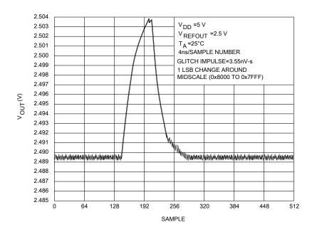
FIGURE 8. Digital to Analog glitch impulse (negative).
